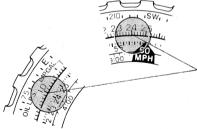
Find the position where the value on the dial ruler scale corresponding to 10 on the bezel ruler scale is the same as the value on the bezel ruler scale corresponding to 57.6 on the dial ruler scale.
